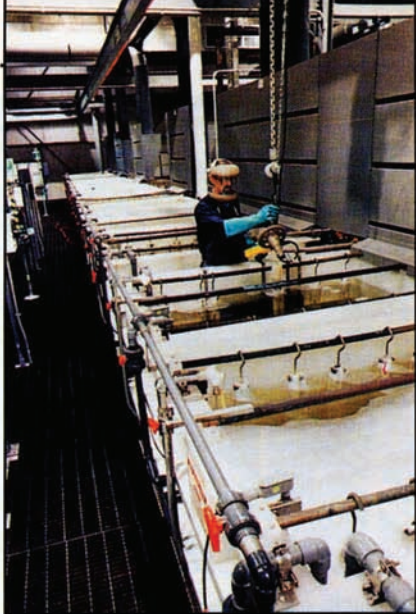
PART IS DIPPED into cadmium plating tank
