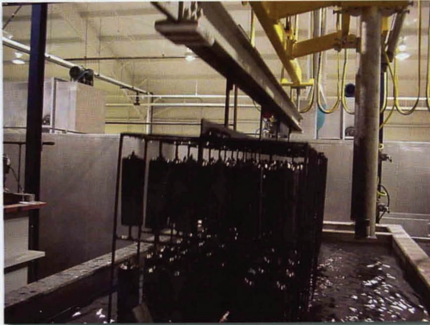
After coating, parts will enter a transfer area, where a trolley will move them into the oven.
